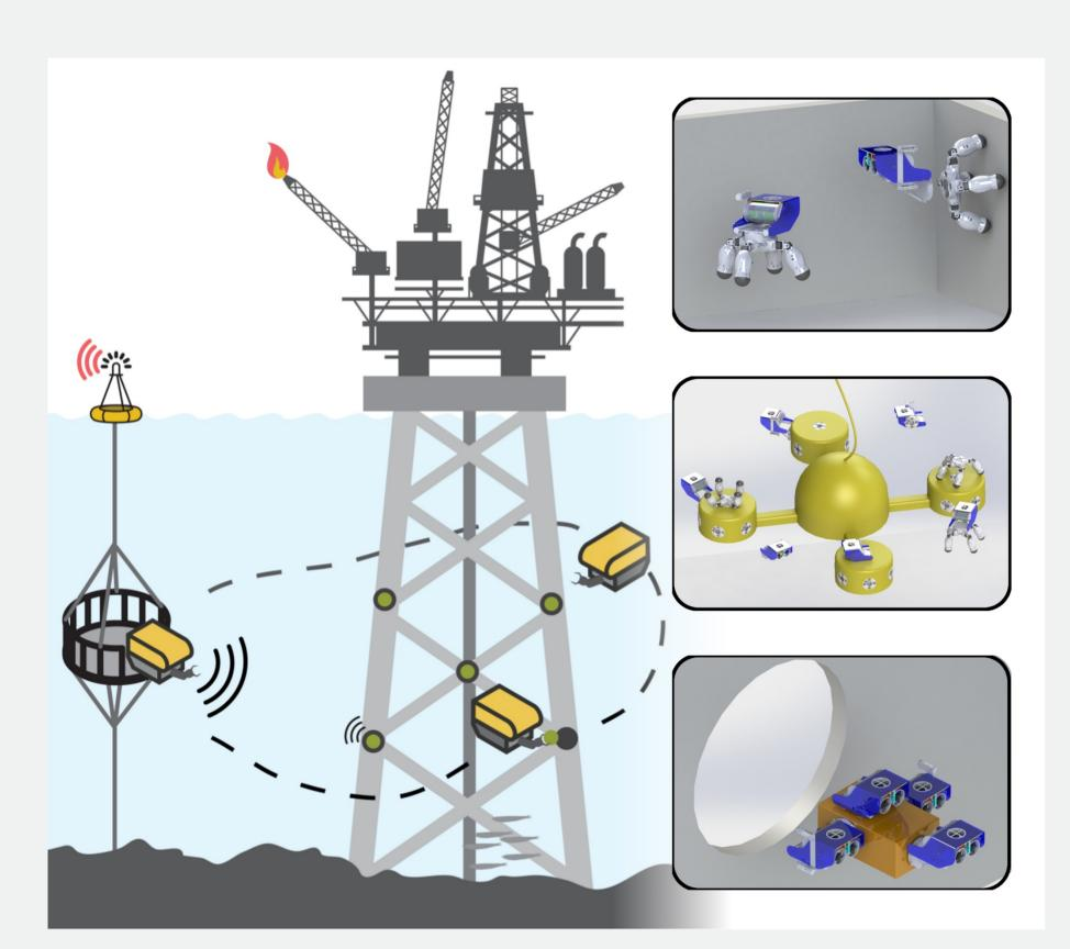
**REMORA Vision** - Concept illustrations of the system during an offshore inspection operation. Multiple robots with different capabilities are deployed to inspect the structure, deliver sensor nodes or retrieve data from previously installed sensors. In between missions, the robots reside at the subsea docking station, where they can recharge batteries, transfer mission data, communicate with on-shore monitoring centre or be repaired.
