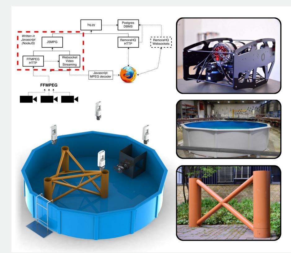
**REMORA Infrastructure** - Software and hardware experimental facilities are currently under implementation. A Python based development environment was implemented to enable rapid deployment of new control and perception functionalities into the individual robots. Further, a scaled model of an offshore platform leg was built to enable experimental validation in quasi-realistic scenario. 8 ROVs are ready for testing ground-breaking ideas in the area of reconfigurable modular robotics.
